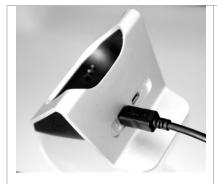
Put your phone on its support. Plug the USB cable into the 5V socket of the desktop charger. Plug the other end of the USB cable into the AC/DC adaptor. Plug the AC/DC adaptor into the mains power supply.
